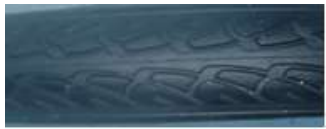
In the picture on the left, the "arrows" point left, giving you direction of rotation.
