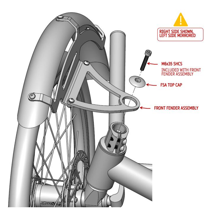
ALIGN FRONT FENDER SO THAT IT IS PARALLEL TO FRONT WHEEL, THEN TIGHTEN TO HEADSET ASSEMBLY
