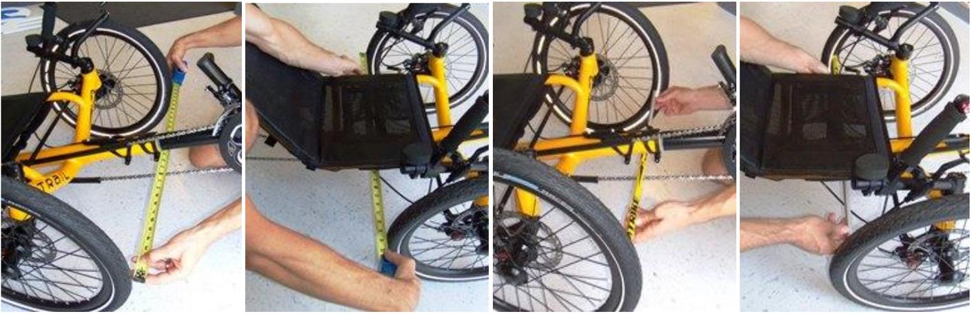
It's very important to get this right...if you have a quarter inch of toe your tires will wear out very quickly and handling performance will be degraded. Proper toe-in will also affect rolling efficiency. Too much toe-in (greater than 1/16" or toe-out where the front of wheel is wider than the rear) are to be avoided as either incorrect setting will significantly reduce rolling efficiency.
