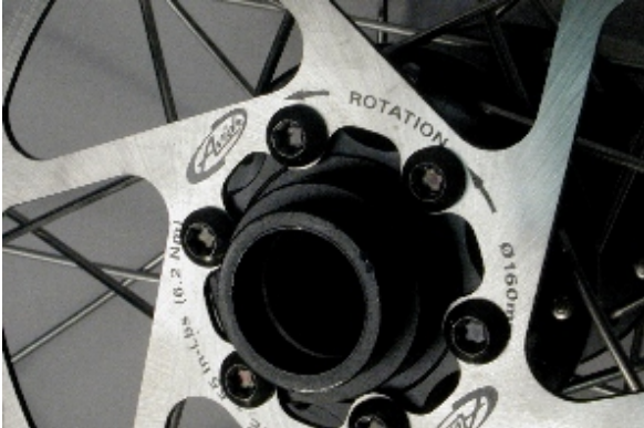
The direction of rotation is written on the brake rotors.
