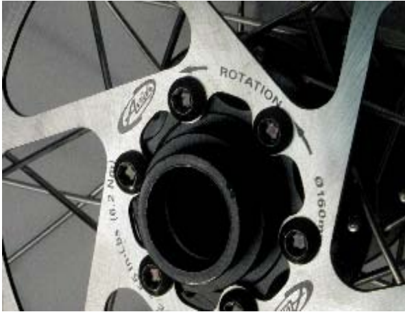
The direction of rotation is indicated on the brake rotors.
